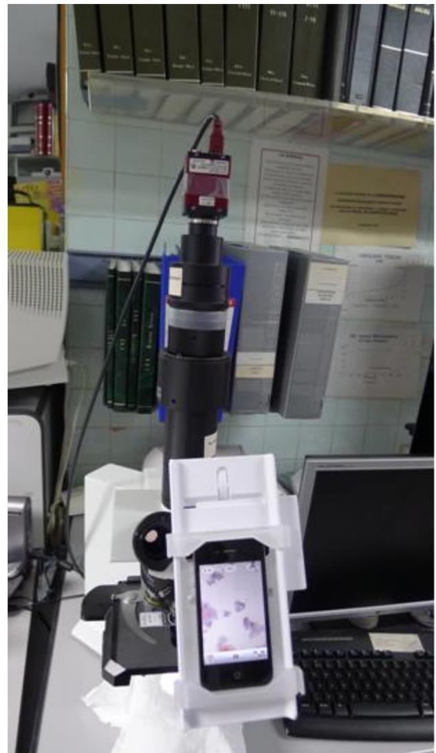
**Figure 3: Skylight® mobile adaptor for the microscope**
